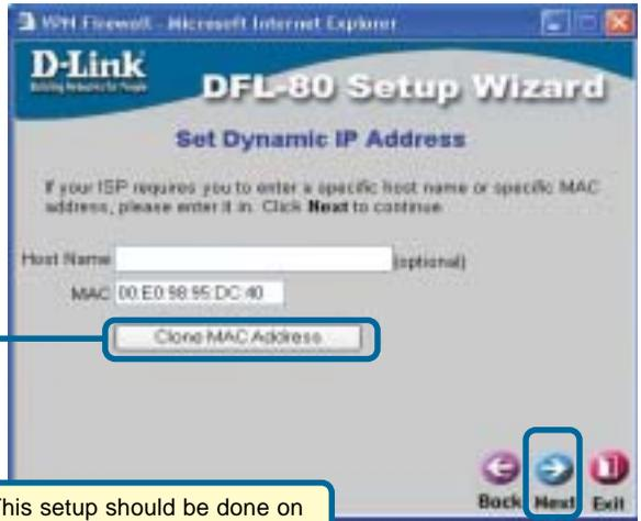
Click the **“Clone MAC Address”** button to automatically copy the MAC address of the network adapter in your computer. You can also manually type in the MAC address.
