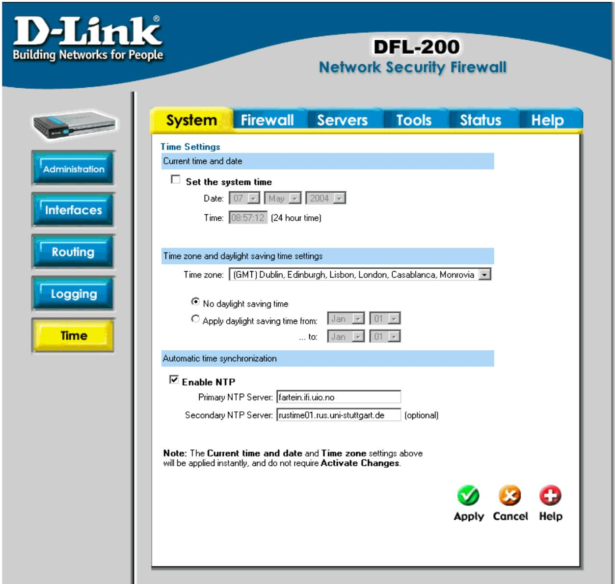
The screenshot shows the D-Link DFL-200 Network Security Firewall configuration interface. The top navigation bar includes 'System', 'Firewall', 'Servers', 'Tools', 'Status', and 'Help'. The left sidebar contains 'Administration', 'Interfaces', 'Routing', 'Logging', and 'Time' (highlighted in yellow). The main content area is titled 'Time Settings' and is divided into three sections:
