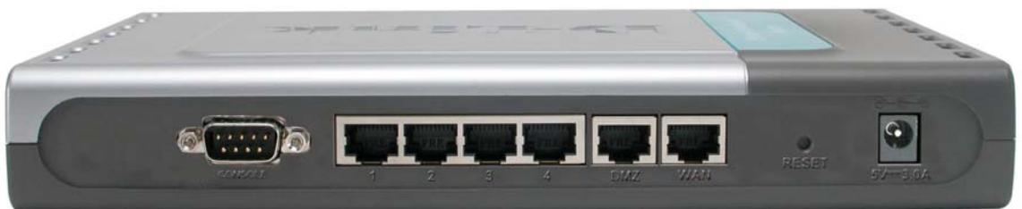
**Console:** Serial access to the firewall software, 9600, 8bit, None Parity, 1Stop bit.
