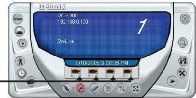
Select any of the four cameras for the View Mode format. If there is a green light next to the camera button that means that the IPView SE has a camera connected.
