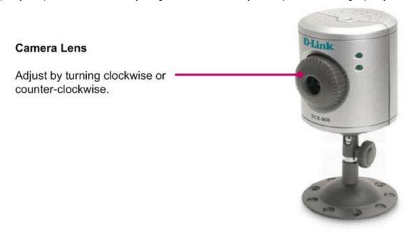
**NOTE:** You can further adjust the Internet Camera's image quality through the Web Configuration under SETUP > Video. Please refer to the Web Configuration section for further details.
