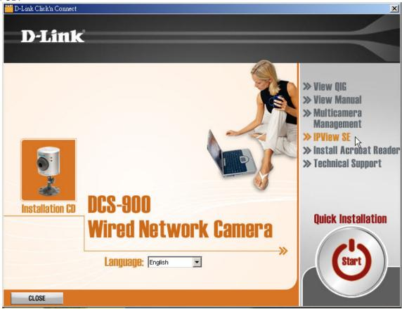
IPView SE software is included for administrators to manage up to 4 DCS-900s remotely. Administrators can also record to hard drive and configure advanced settings for the DCS-900. IPView SE is a complete software management tool for the DCS-900 and includes all configurable settings available in the web configuration utility.
