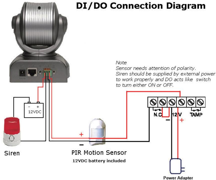
The above diagram shows a typical wiring configuration for a normally closed PIR motion sensor. Please refer to your specific motion sensor for the power supply connection to the device since this will be critical to the success of your installation. Note that the positive from the PIR is connected to the D+ of the I/O port of the camera and the negative from the PIR is connected to the D- of the camera I/O port.
