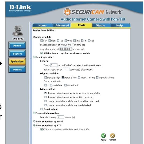
In this window, follow the steps below to set the application settings for snapshots to be sent to your email account or FTP server when triggered by a motion sensor or other external device:
