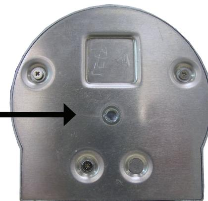
**Note:** Located on the bottom panel of the DCS-5300, the socket is used to connect the camera stand to the Network Camera by attaching the screw head on the camera stand to the Network Camera.
