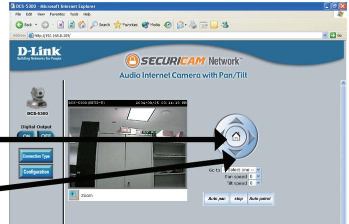
**Pull down menu:** Select a preset position to move the camera to.
