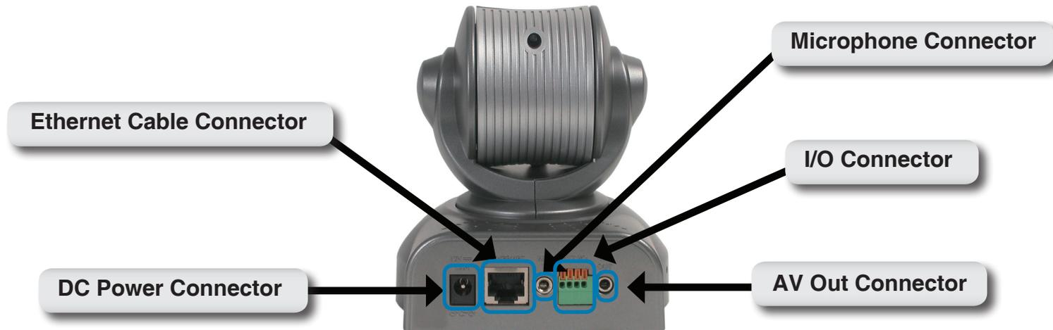
**Ethernet Cable Connector** - The DCS-5300 back panel features an **RJ-45** connector for connections to 10Base-T Ethernet cabling or 100Base-TX Fast Ethernet cabling. This network port supports the **NWay protocol**, allowing the Network Camera to automatically detect or negotiate the transmission speed of the network.
