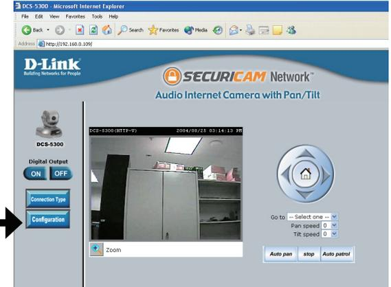
There are 5 tabs across the top of the **Configuration** screen. From each tab, different elements of the DCS-5300 can be configured. The **Advanced** tab is the default screen in **Configuration** and **Network** is the default screen under **Advanced**.
