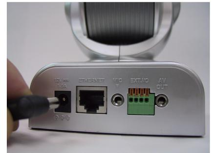
When you have a proper connection, the LED will turn from **red** to **green**. If you are directly connected to the camera via a crossover cable, the light may cycle on and off and your computer may show an intermittent loss of connectivity. This is normal until you have configured your Network Camera.
