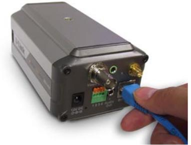
Locate the antennas included with your DCS-3420 and attach them to the antenna connectors located on the back of the DCS-3420.
