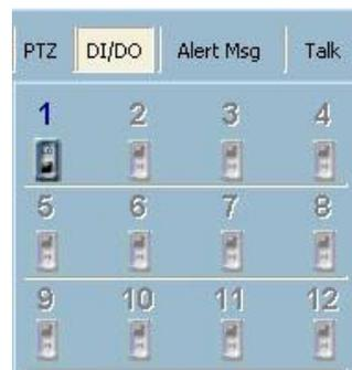
Clicking on the “DI/DO” button shown below, you can switch to the DI/DO controls. The color of the channel number indicates the status of the camera’s DI (Digital Input). You can click the “Switch button” to change the HI/LOW state of the DO (Digital Output). With these features, you can monitor the remote sensor input from DI and also trigger the camera by DO switch.
