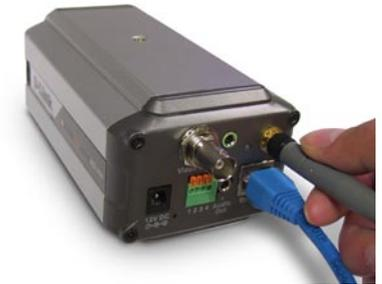
Attach the external power supply to the DC power input connector located on the Internet Camera's back panel (labeled 12VDC) and connect it to your wall outlet.
