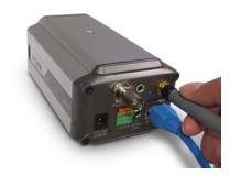
Attach the external power supply to the DC power input connector located on the Internet Camera's back panel (labeled 12VDC) and connect it to your wall outlet.
