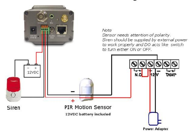
The above diagram shows a typical wiring configuration for a normally closed PIR motion sensor. Please refer to your specific motion sensor for the power supply connection to the device since this will be critical to the success of your installation. Note that the positive from the PIR is connected to the D+ of the I/O port of the camera and the negative from the PIR is connected to the D- of the camera I/O port.
