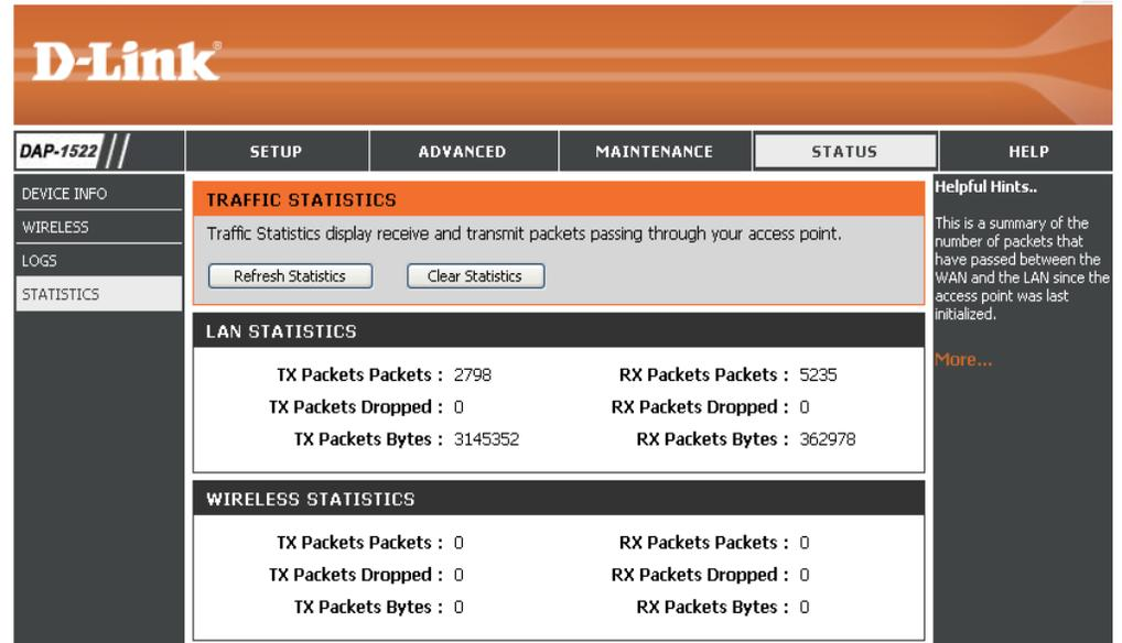
The screenshot shows the D-Link web interface for the DAP-1522 device. The top navigation bar includes tabs for SETUP, ADVANCED, MAINTENANCE, STATUS, and HELP. The left sidebar contains links for DEVICE INFO, WIRELESS, LOGS, and STATISTICS. The main content area is titled "TRAFFIC STATISTICS" and includes a description: "Traffic Statistics display receive and transmit packets passing through your access point." Below this are two buttons: "Refresh Statistics" and "Clear Statistics".
