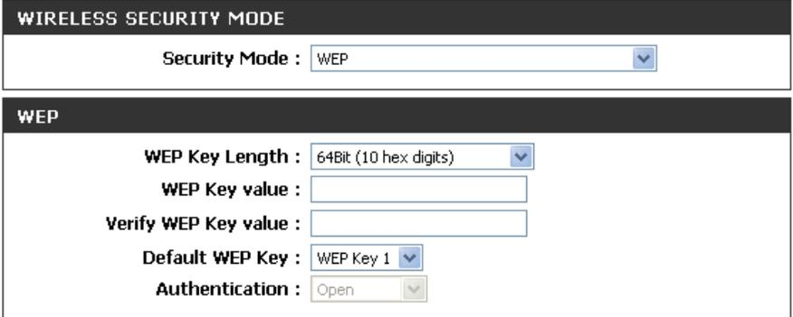
The screenshot shows the configuration interface for WEP. It is divided into two sections: 'WIRELESS SECURITY MODE' and 'WEP'. In the 'WIRELESS SECURITY MODE' section, 'Security Mode' is set to 'WEP'. In the 'WEP' section, 'WEP Key Length' is set to '64Bit (10 hex digits)'. There are two empty text input fields for 'WEP Key value' and 'Verify WEP Key value'. 'Default WEP Key' is set to 'WEP Key 1' from a dropdown menu. 'Authentication' is set to 'Open' from a dropdown menu.
