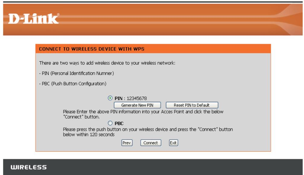
Start WPS on the wireless device you are adding to you wireless network to complete the setup.
