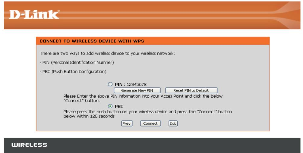
Press down the Push Button on the wireless device you are adding to your network to complete the setup.
