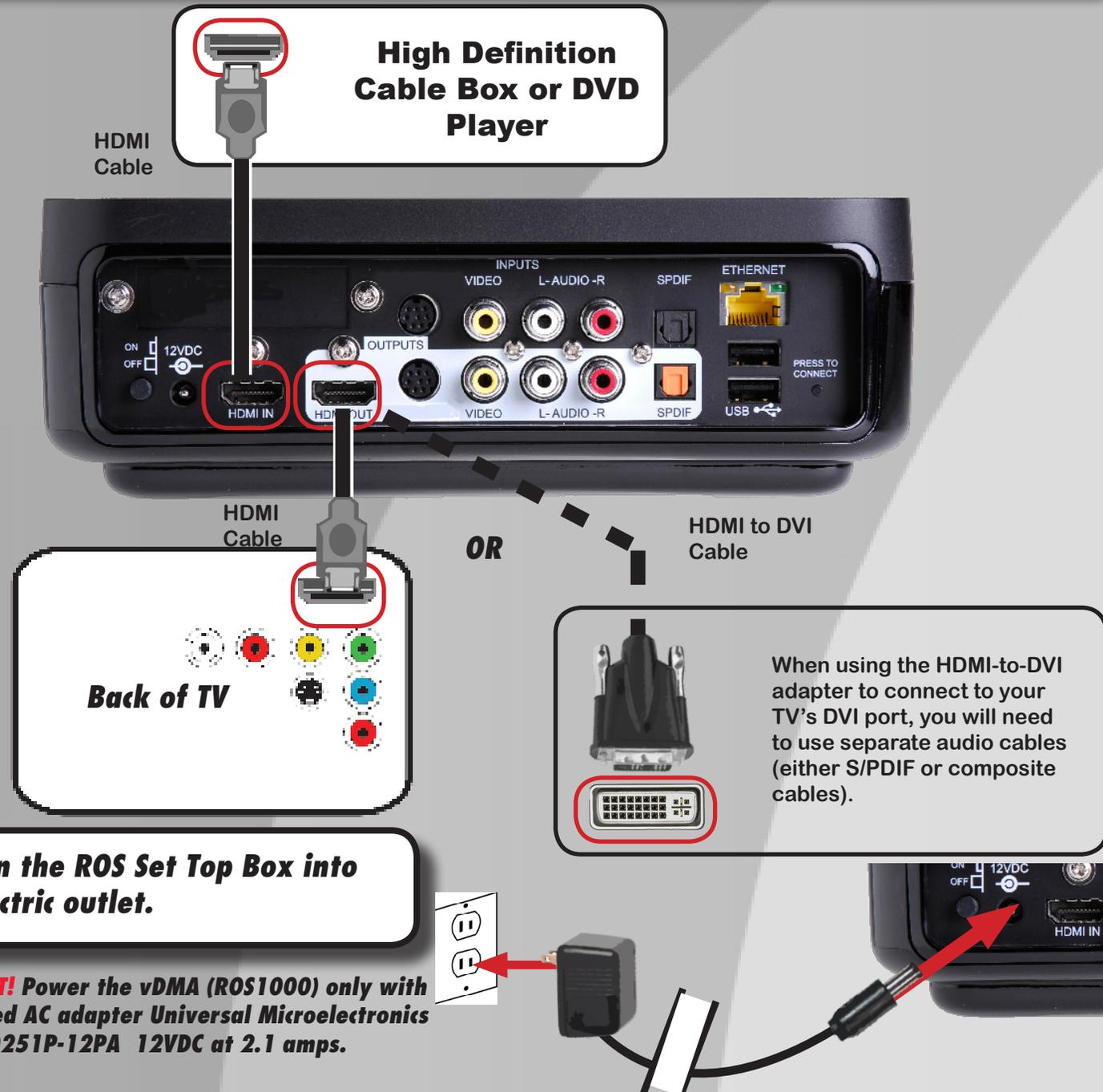
**IMPORTANT!** Power the vDMA (ROS1000) only with the included AC adapter Universal Microelectronics model UP0251P-12PA 12VDC at 2.1 amps.
