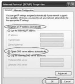
Select the options "Obtain an IP address automatically" and "Obtain DNS server address automatically".
