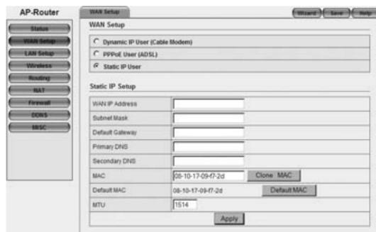
2. Under "WAN Setup" select "Static IP User". This setting is for providers who use a fixed Static IP address.
