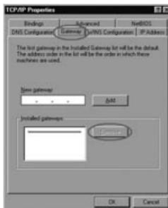
Under the tab "Gateway", the list of "Installed gateways" must be empty. If so required, select each gateway and click "Remove".
