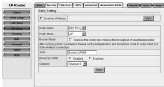
The default SSID is "Sweex LW055". We recommend not changing this so you can always recognise the router. Here you can also find other options such as "Channel" and "Radio Mode". We again recommend maintaining the default values. You can enable or disable the wireless part under "Disabled Wireless". This feature is enabled by default.
