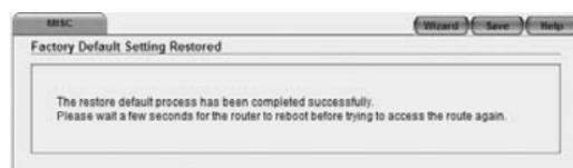
After one minute, the router can be accessed via the default IP address (192.168.55.1).
