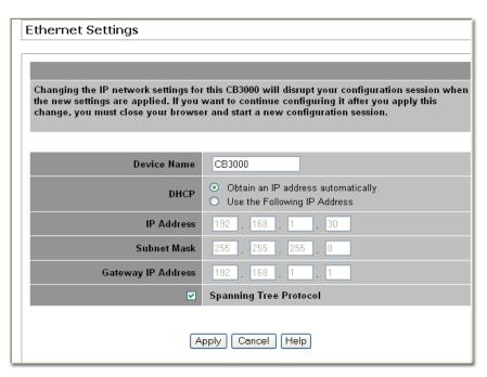
2. Configure the **Ethernet Settings** screen to assign a device name and set network address information the CB3000 uses to
