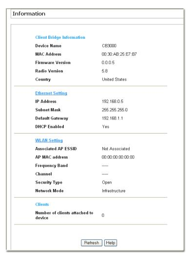
The **Information** screen displays high level device name and network address information. The page is read-only with no configurable data fields. The CB3000 is now ready to have its WLAN settings configured, then its Ethernet Settings. For more information, see *Configuring CB3000 WLAN Settings on page -13* and *Configuring CB3000 Ethernet Settings on page -16*.
