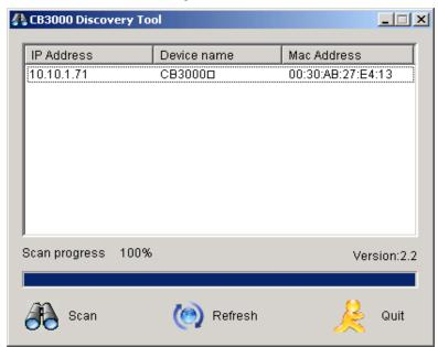
The **CB3000 Discovery Tool** screen displays and automatically begins a device search for other CB3000's.
