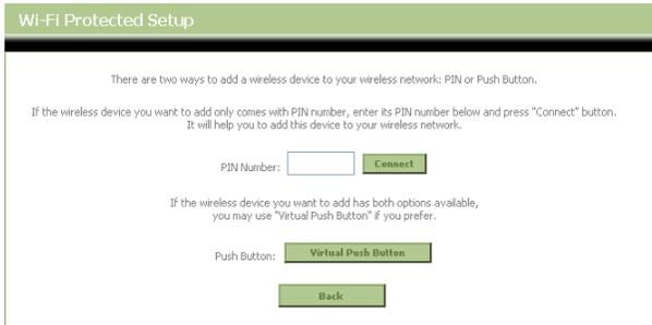
In this Wizard, you can activate the Pin Code feature. To start with the Pin Code authentication, you need the Pin Code generated by your Wireless Client.
