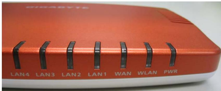
The table below describes the LED indicators on the front panel of the Router.
