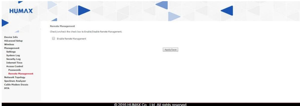
**Enable Remote Management:** Check to allow remote management. To access your router remotely from a web browser, enter the *WAN IP address:8080*.
