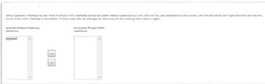
Without gateway interface (or can have multiple WAN interfaces) used as system default gateways but only one will be used according to the priority with the first being the highest and the last one the lowest if the WAN interface is connected. Priority order can be changed by removing all and adding them back in again.
