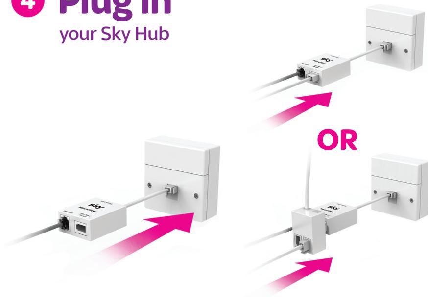
1. Plug the white end of the microfilter with the grey ADSL cable attached directly into your master phone socket.
