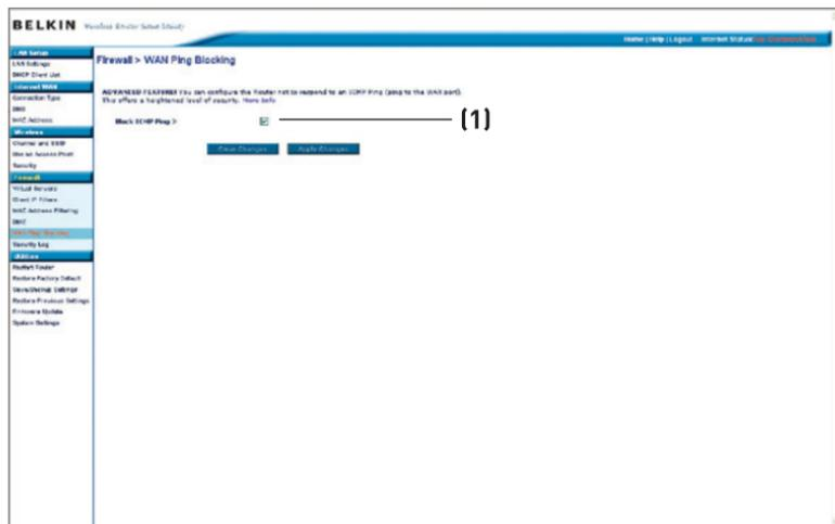
To turn off the ping response, select “Block ICMP Ping” (1) and click “Apply Changes”. The Router will not respond to an ICMP ping.
