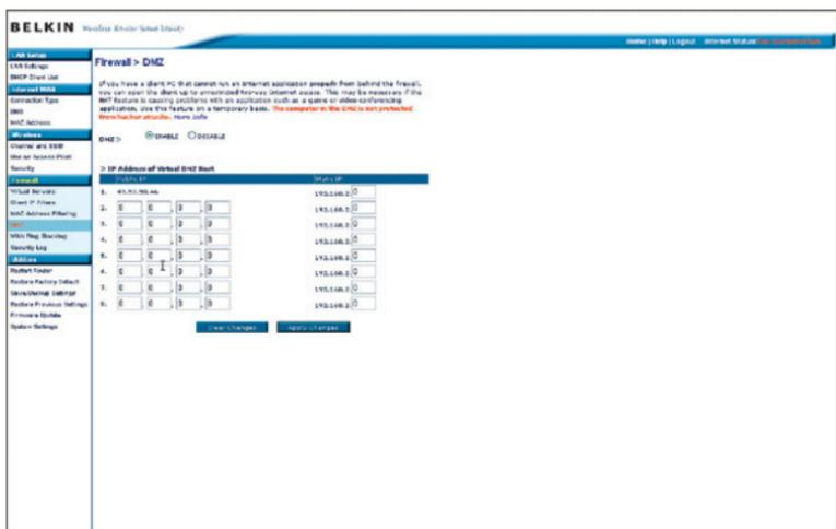
To put a computer in the DMZ, enter the last digits of its IP address in the IP field and select “Enable”. Click “Apply Changes” for the change to take effect.
