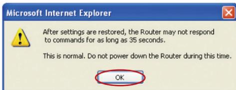
4. A 35-second countdown will appear on the screen. When the countdown reaches zero, the Router’s configuration will be restored. The Router’s home page should appear automatically. If not, type in the Router’s address (default = 192.168.2.1) into the navigation bar of your browser.
