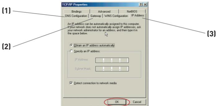
3. If “Specify an IP address” is selected, your Router will need to be set up for a static IP connection type. Write the address information in the table below. You will need to enter this information into the Router.
