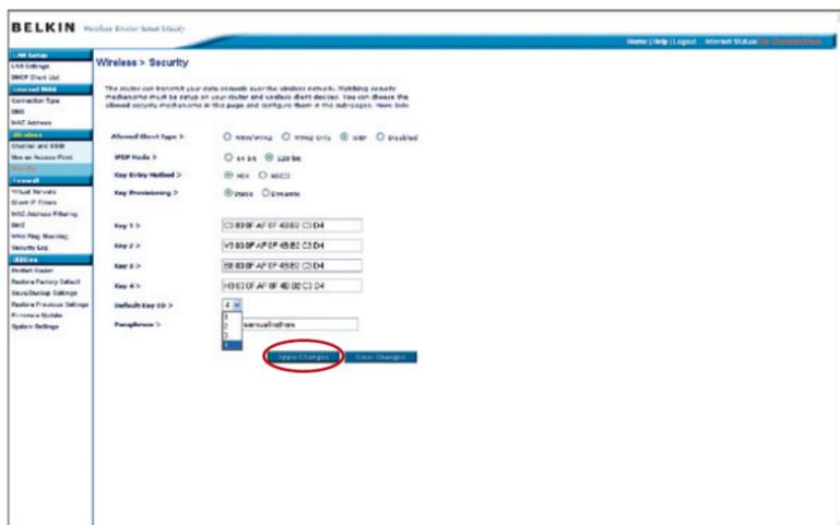
**WARNING:** If you are configuring the Wireless G Router or access point from a computer with a wireless client, you will need to ensure that security is turned on for this wireless client. If this is not done, your client will lose its wireless connection.
