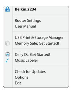
The Belkin Router Manager appears in your system tray (Windows) or menu bar (Mac). Its icon indicates the current status of your Router and also allows you to access your Router's settings to make changes. It also provides quick access to software that came bundled with your Router.
