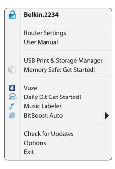
The Belkin Router Manager appears in your system tray (Windows) or menu bar (Mac). Its icon indicates the current status of your Router and also allows you to access your Router's settings to make changes. It also provides quick access to software that came bundled with your Router.
