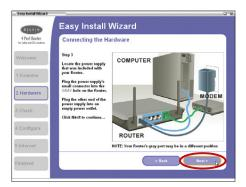
2.3 This step instructs you to locate the power supply that is included with your Router. Plug the power supply's small connector into the GRAY port on the Router. Plug the power supply into an empty power outlet. Click "Next" to continue.
