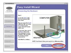
2.2 This step instructs you to locate the BLUE cable that is included with your Router. Plug one end of this cable into ANY one of the BLUE ports on your Router. Plug the other end of the cable into the networking port on your computer. Click "Next" to continue.
