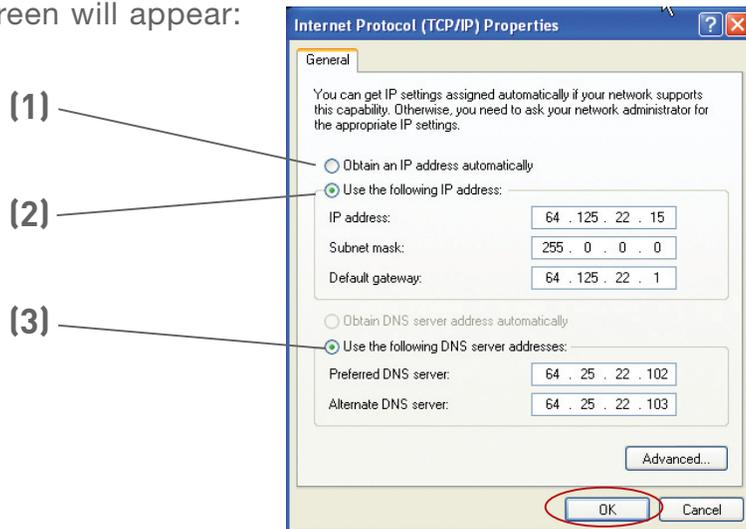
5. If "Use the following IP address" (2) is selected, your Router will need to be set up for a static IP connection type. Write the address information in the table below. You will need to enter this information into the Router.
