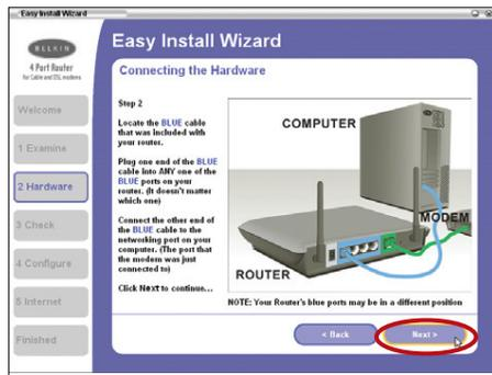
2.2 This step instructs you to locate the BLUE cable that is included with your Router. Plug one end of this cable into ANY one of the BLUE ports on your Router. Plug the other end of the cable into the networking port on your computer. Click "Next" to continue.
