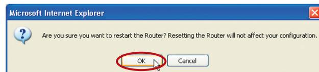
3. The following message will appear. Restarting the Router can take up to 60 seconds. It is important not to turn off the power to the Router during the restart.
