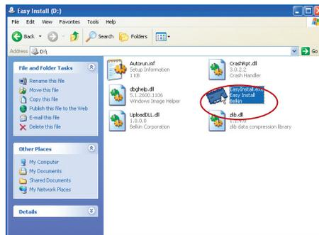
4. If the Easy Install Wizard is still does not start, reference the section titled “Manually Configuring Network Settings” (page 89 of this manual for alternative setup method).
