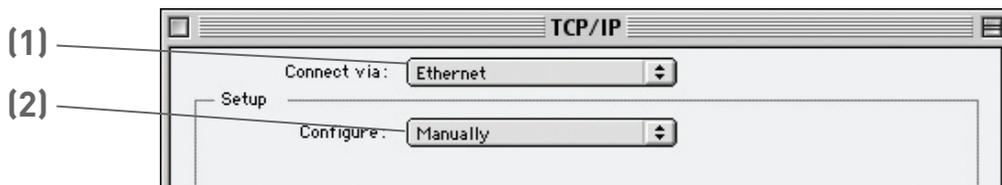
3. Next to "Configure" (2), if "Manually" is selected, your Router will need to be set up for a static IP connection type. Write the address information in the table below. You will need to enter this information into the Router.
