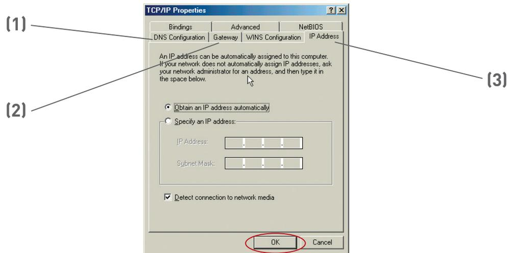
3. If “Specify and IP address” is selected, your Router will need to be set up for a static IP connection type. Write the address information in the table below. You will need to enter this information into the Router.
