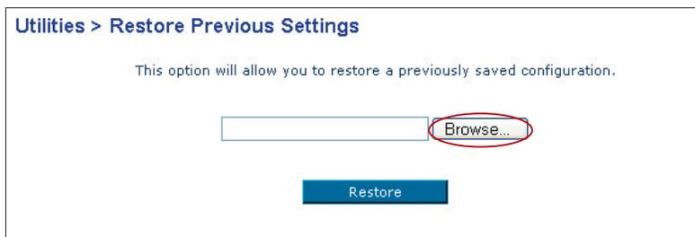
1. Click "Browse". A window will open that allows you to select the location of the configuration file. All configuration files end with a ".bin". Locate the configuration file you want to restore and double-click on it.
