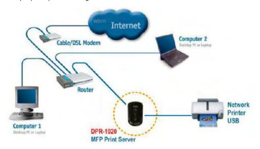
**WARNING:** Only a USB printer may be connected to the USB port of the DPR-1040. Do not connect any other USB devices to the USB port of the DPR-1040; to do so, may damage the unit and will void the warranty for this product.
