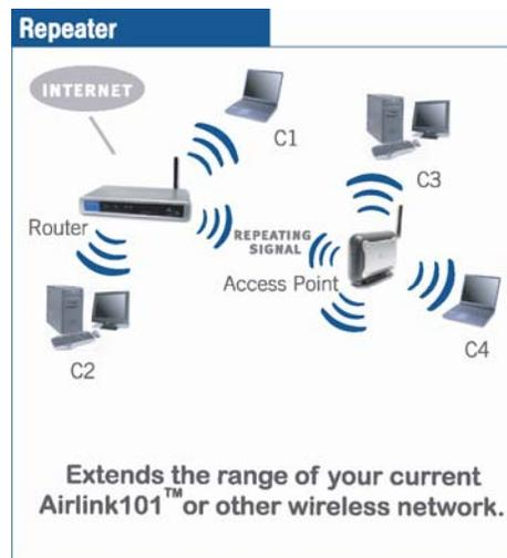
**Note:** The repeater mode may not be compatible with all routers due to the lack of a standard protocol for repeater mode.
