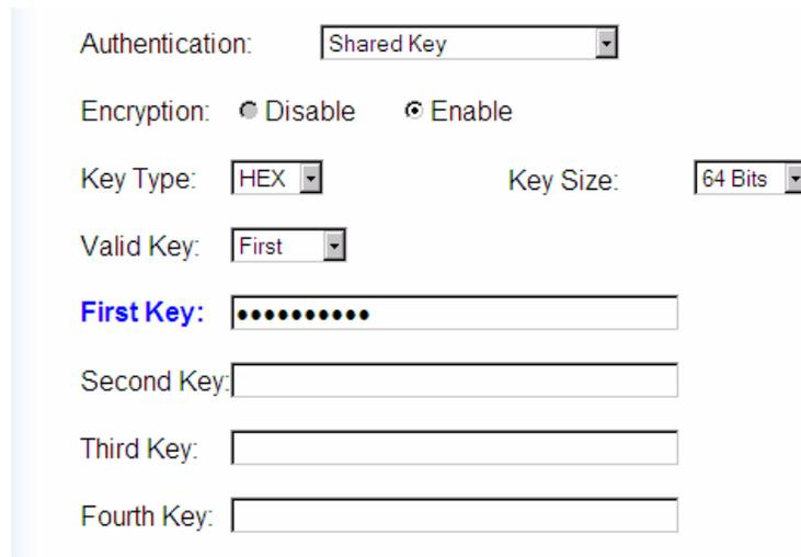
The screenshot shows a configuration interface for WEP. It includes a dropdown menu for 'Authentication' set to 'Shared Key', radio buttons for 'Encryption' with 'Enable' selected, a dropdown for 'Key Type' set to 'HEX', and a dropdown for 'Key Size' set to '64 Bits'. Below these are four key input fields: 'Valid Key' (set to 'First'), 'First Key' (filled with 10 dots), 'Second Key', 'Third Key', and 'Fourth Key'.
