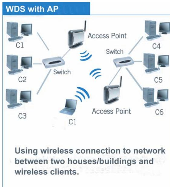
If you want to use the AP431W as an Access Point with minimal configuration, just connect it to your existing router or switch with a Cat. 5 network cable and then power it on. The Access Point is ready to use with its default settings:
