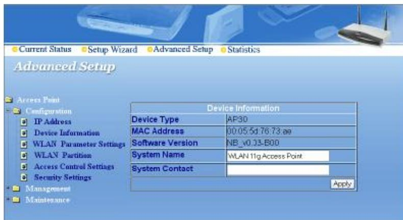
The screenshot shows the 'Advanced Setup' interface with a navigation menu on the left and a 'Device Information' table on the right. The navigation menu includes 'Access Point', 'Configuration', 'Management', and 'Maintenance'. Under 'Configuration', there are sub-menus for 'IP Address', 'Device Information', 'WLAN Parameter Settings', 'WLAN Partition', 'Access Control Settings', and 'Security Settings'. The 'Device Information' table contains the following fields:
