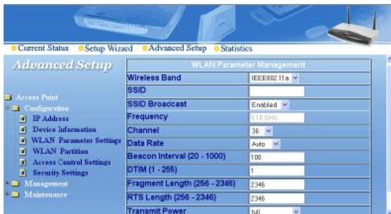
The screenshot shows the 'Advanced Setup' interface with a navigation menu on the left and a 'WLAN Parameter Management' table on the right. The navigation menu is identical to the previous screenshot. The 'WLAN Parameter Management' table contains the following fields:
