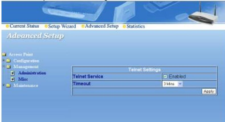
**Telnet Service:** When enabled, Administrator can access the device configuration via Telnet operation.
