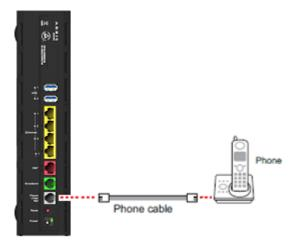
• For two phones, connect the phone cable to a splitter and then to the phones.
