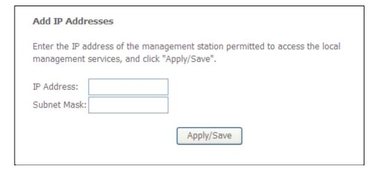
Input the IP Address and Subnet Mask which you want to configure, and then click **Apply** to enable this IP Address.
