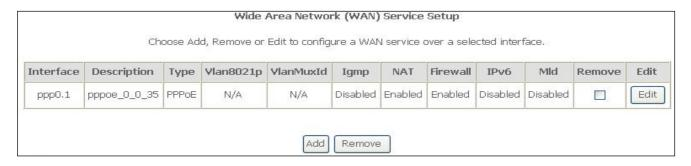
The **WAN Service Interface Configuration** Configuration window allows select a layer 2 interface for this service. Click the **Next** button to continue
