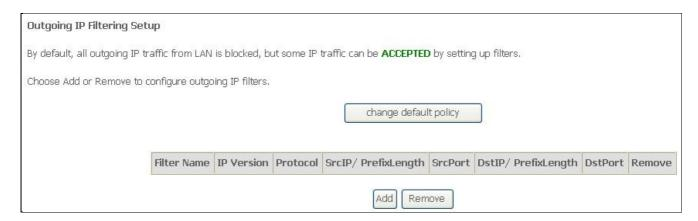
Enter the information in the section. Explanations of parameters are described below. Click the **Apply / Save** button to add the entry in the Active Outbound IP Filtering table.
