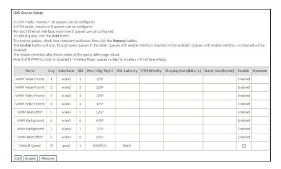
This window allows you to configure a QoS queue entry and assign it a specific network interface.
