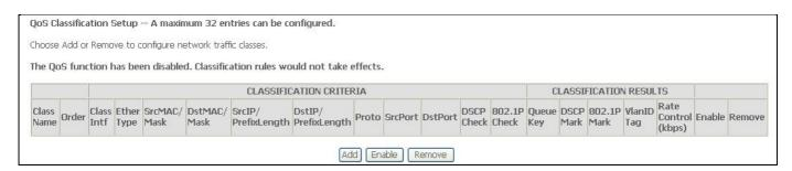
Use this window to create a traffic class rule to classify the upstream traffic, assign a queue that defines the precedence and the interface, and optionally overwrite the IP header DSCP byte. A rule consists of a class name and at least one condition. Please remember that all of the specified conditions on this window must be met for the rule to take effect. Click the **Apply / Save** button to save and activate this rule.
