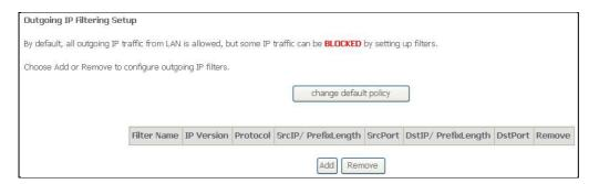
Now default policy is ACCEPT, it means all outgoing IP traffic from LAN is allowed, but some IP traffic can be blocked by setting up filters.
