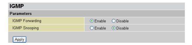
IGMP Forwarding: Accepting multicast packet. Default is set to Enable.
