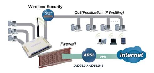
Figure 1.1 Application Diagram of TW-EA510v4
