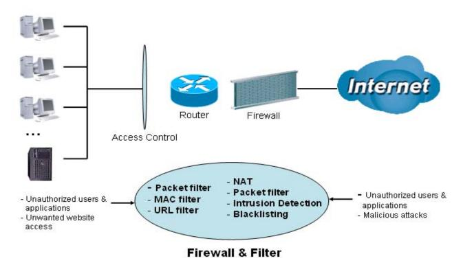
**Firewall**: Prevents access from outside your network. The router provides three levels of security support:
