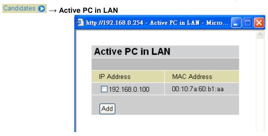
Active PC in LAN displays a list of individual Ethernet device's IP Address & MAC Address which connecting to the router.
