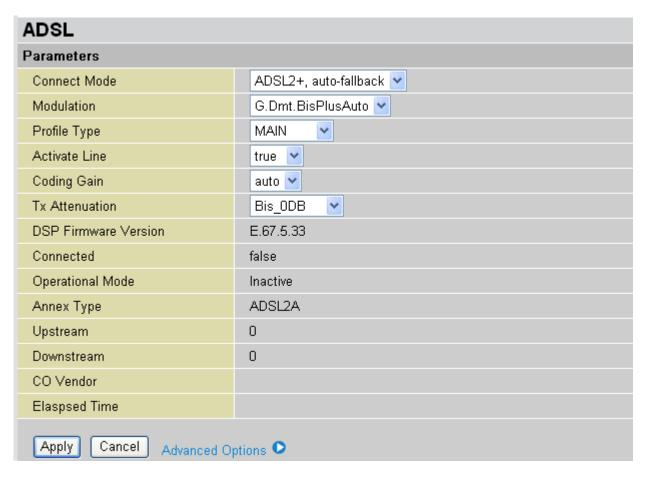
**Connect Mode:** This mode will automatically detect your ADSL line code, ADSL2+, ADSL2, G.dmt, G.lite, T1.413, AnnexM2 and AnnexM2+. But in some area, multimode cannot detect the ADSL line code well. If it is the case, please adjust the ADSL line code to G.dmt or T1.413 first. If it still fails, please try the other values such as ALCTL, ADI, etc. If you still having trouble with the line, please check with your ISP for line connect information.
