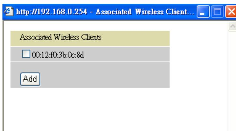
Associate Wireless Client displays a list of individual wireless device's MAC Address that currently connects to the router.
