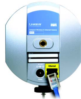
Figure 4-1: Connect the Ethernet Network Cable
