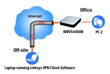
Figure 3-2: Computer to VPN Router
