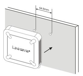
Figure 5-8: Wall Mounting Hardware
