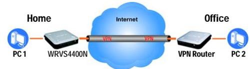
Figure 3-1: VPN Router to VPN Router
