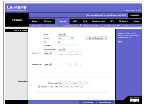
Figure 6-33: Firewall - Edit IP ACL Rule
