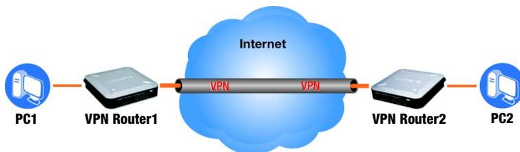
Figure C-1: Diagram of Gateway-to-Gateway VPN Tunnel
