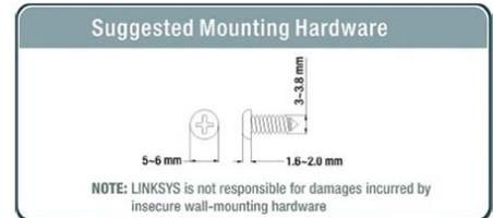
**Figure 5-7: Mounting Dimensions**
