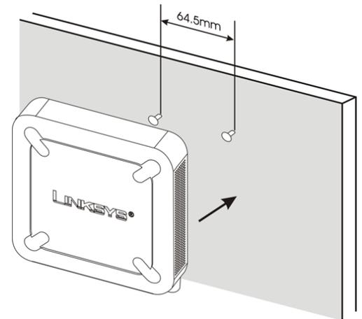
**Figure 5-8: Wall Mounting Hardware**
