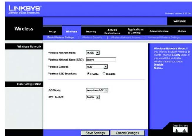
Figure 5-16: Wireless Tab - Basic Wireless Settings
