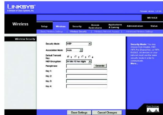
**Figure 5-19: Wireless Tab - Wireless Security (WEP)**
