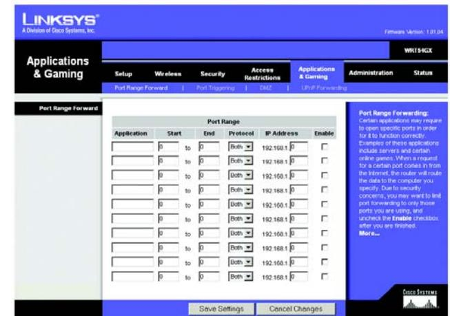
Figure 5-28: Applications and Gaming Tab - Port Range Forward
