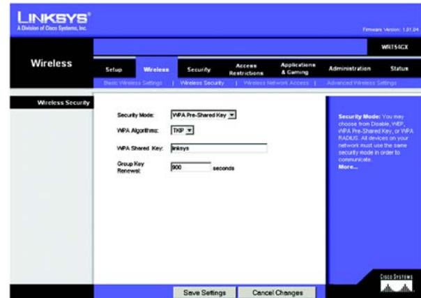
Figure 5-17: Wireless Tab - Wireless Security (WPA Pre-Shared Key)
