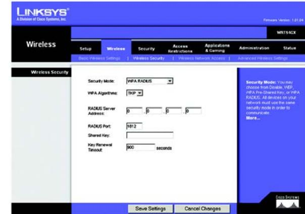
Figure 5-18: Wireless Tab - Wireless Security (WPA RADIUS)
