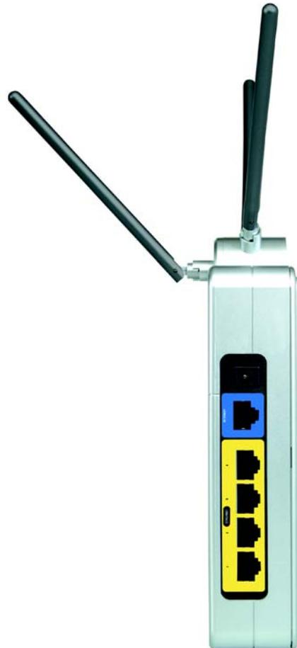
Figure 3-1: The Router's Back Panel
