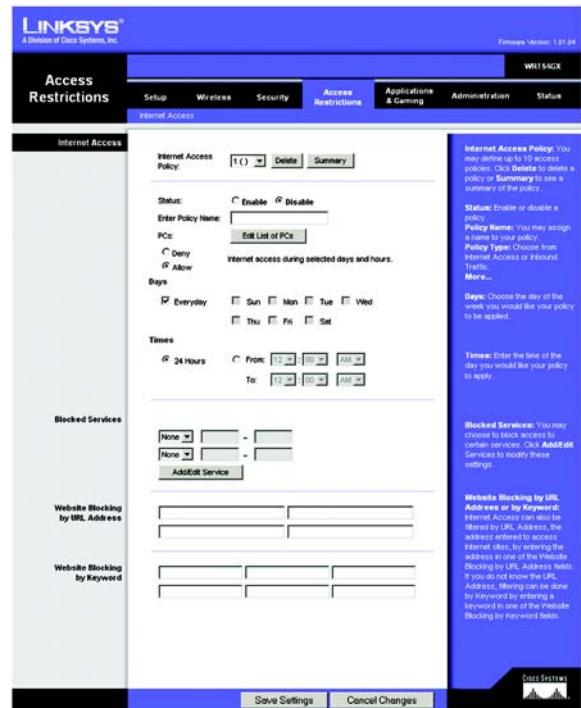
Figure 5-24: Access Restrictions Tab - Internet Access
