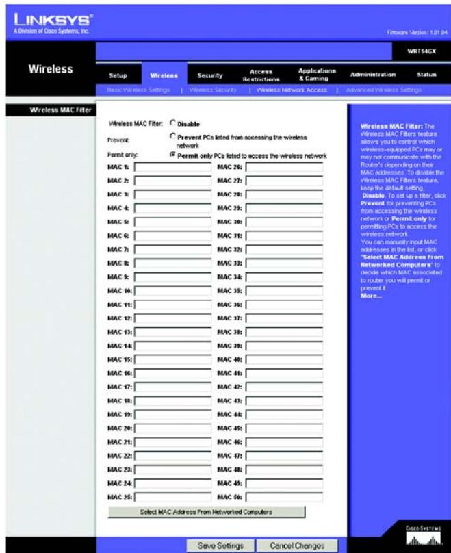
Figure 5-20: Wireless Tab - Wireless MAC Filter
