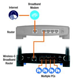
Figure 4-5: Diagram for Connection to Another Router
