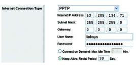
Figure 5-6: PPTP Connection Type
