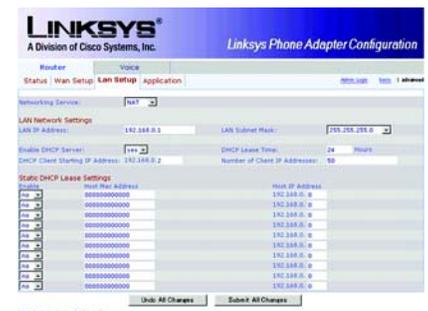
Figure 6-6: Router - LAN Setup Screen
