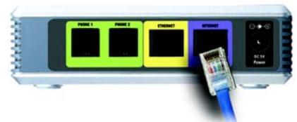
**Figure 4-3: Connect to the Modem**
