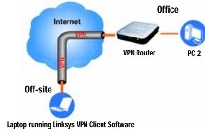
Figure 3-2: Computer to VPN Router
