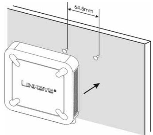
Figure F-3: Wall-Mounting the Router
