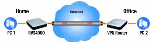
Figure 3-1: VPN Router to VPN Router
