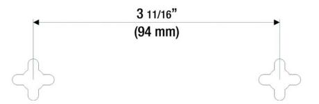
Figure D-4: Wall-Mounting Hardware
