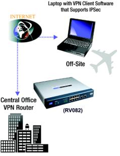
Figure 2-2: Computer-to-VPN Router VPN
