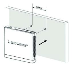
Figure D-3: Wall-Mounting the Router
