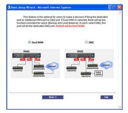
Figure 5-61: Basic Setup Wizard -Dual WAN or DMZ
