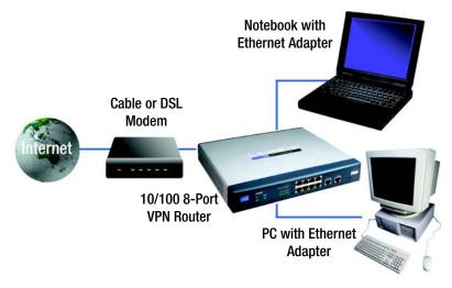
Figure 4-1: Example of a Typical Network
