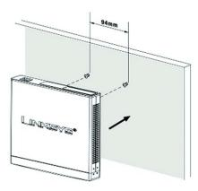
Figure D-3: Wall-Mounting the Router
