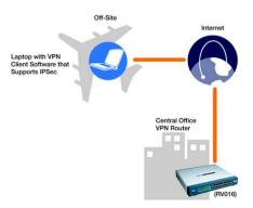
Figure 2-2: Computer-to-VPN Router VPN
