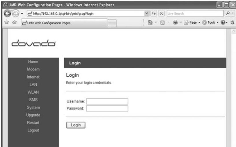
Once you have connected a computer with either an Ethernet cable or by Wireless LAN, open your web browser and access the following website:
