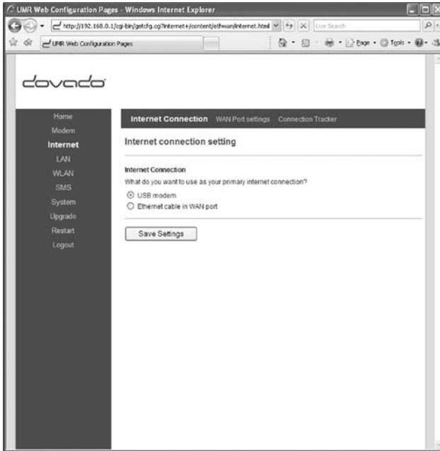
The UMR can also be used with a regular fixed broadband connection from an ADSL- or Cable-modem. To select your primary broadband connection, push **Internet** and then select **Internet Connection**. Make your selection and then push **Save Settings**.
