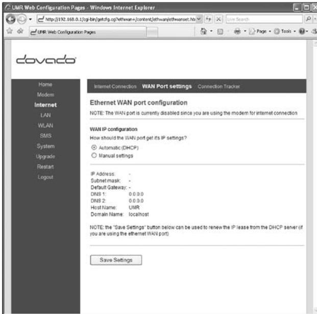
The default setting is that your operator automatically will give you an IP address, should your operator have given you a static (specific) IP address than select **Manual settings** and fill in the given information in the relevant fields.
