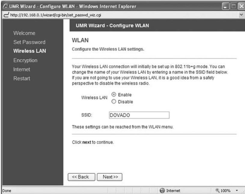
If you do not have any devices using Wireless LAN, choose disable for the Wireless LAN option, and then click on **Next** to continue (this will skip the encryption page). If you have a device using wireless LAN, enable Wireless LAN. You can also change the SSID, which is displayed in the client when a network search is performed. When you are done, click on **Next** to continue.
