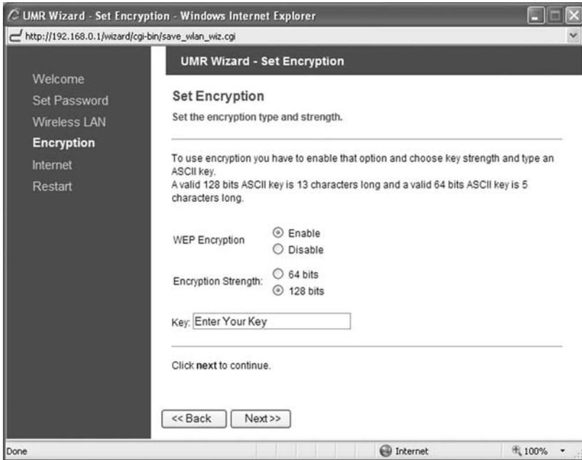
Here you can activate encryption if you would like to restrict access of wireless users onto your private network. Choose **Enable** to enable encryption, it is recommended that you select 128 bits as **Encryption Strength** and then type in a key. The key is needed by all Wireless LAN clients to access your private network. Click on **Next** to continue.
