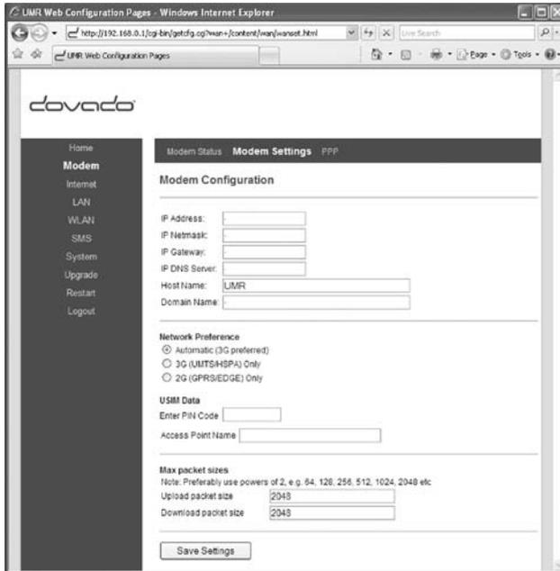
On the **Modem>Modem Settings** page, you will be able to insert all the valid inputs in order to access the internet via your mobile operator. There are several relevant bits of information which are necessary in order to complete this task successfully:
