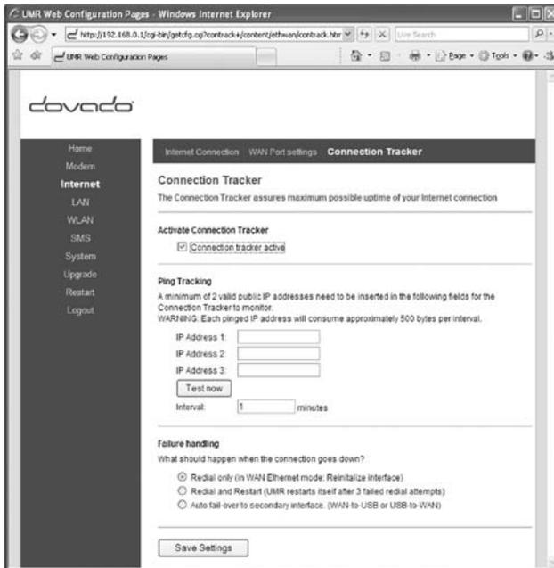
In order to ensure maximum internet availability you can use the Connection Tracker feature. When inserting a minimum of 2 IP addresses, these addresses will be "pinged" with an interval that you specify in minutes in the **Interval** field.
