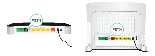
3 Plug the other end of the cable into the **Phone** output port of your filter/splitter.
