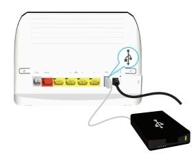
By using a USB hub, you can connect up to five USB mass storage devices to the Technicolor Gateway.
