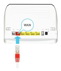
3 Plug the other end of the cable into the Ethernet port of your Internet gateway/modem.
