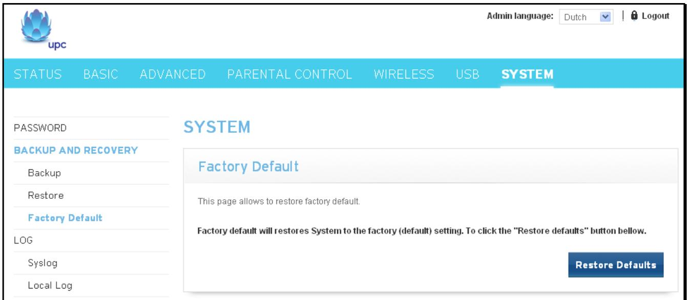
Fig.2-48 System\Backup and Recovery\Factory Default
