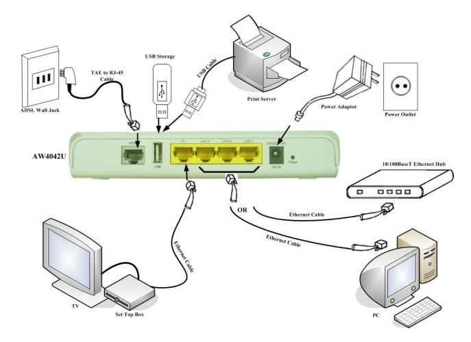
Figure 1.3. Overview of Hardware Connections
