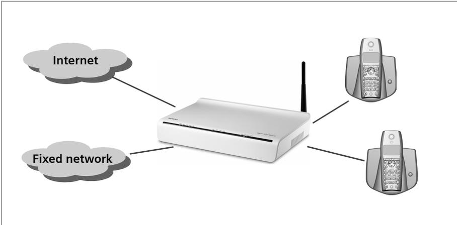
You can choose whether to connect any two analogue phones, a fax machine or an answering machine to the phone ports. You can configure these ports using the Giga762SX WLAN dsl.
