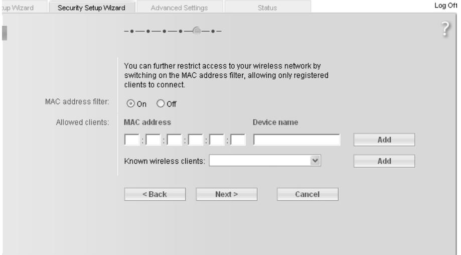
Access control is disabled by default. This means that all PCs that use the correct [SSID](#) can be logged in.
