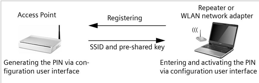
WLAN adapters without WPS can also be set up manually, i.e. the SSID and key must be entered manually. How you can find out which SSID and which pre-shared key is set, you can read in chapter "Configuring wireless connections" on page 85.
