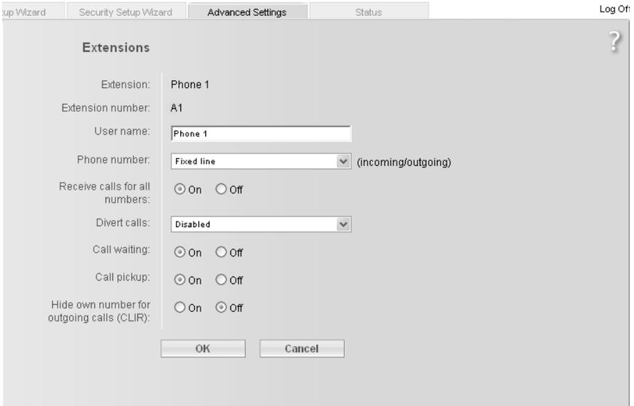
The Extension shows either the selected port of the Giga762SX WLAN dsl (Phone 1 or Phone 2) or the SIP client. The **Extension number** for the extension is preset and is displayed as a call number.
