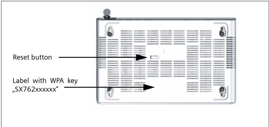
**Reboot function:** Press and hold the right end of the button for more than 1 second but less than 5 seconds to reboot the device. This does not affect the configuration settings.
