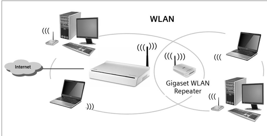
PCs to be connected in a wireless local area network via a repeater must be equipped with an integrated wireless network adapter or you have to connect an external wireless network adapter (e.g. a USB adapter).
