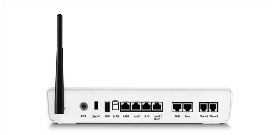
The rear panel of the Giga762SX WLAN dsl houses the ports.
