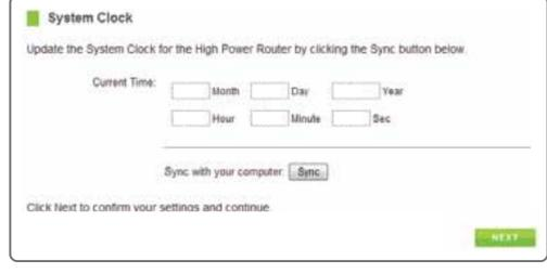
The System Clock is used for system logs and setting schedules for Internet access. Click **Sync** to synchronize the System Clock with the time on your computer.
