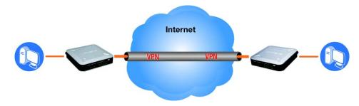
Diagram of Gateway-to-Gateway VPN Tunnel
