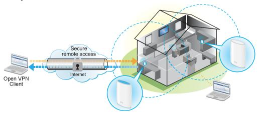
Figure 13. VPN provides a secure tunnel between your home network and a remote computer
