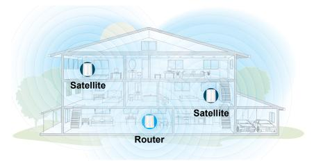
Figure 10. Multilevel house with two Orbi satellites
