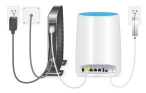
**Note:** The router shown in this image is the Orbi router (model RBR50). The same setup applies to all Orbi routers.
