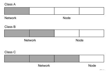
Figure 6-3: Three Main Address Classes
