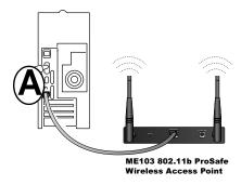
Figure 3-2: Connecting the ME103 to a PC
