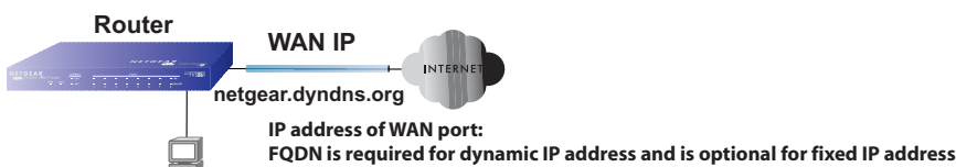
Figure 3-3: Inbound traffic to single WAN port case
