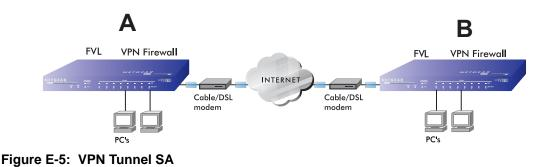
The SA contains all the information necessary for gateway A to negotiate a secure and encrypted communication stream with gateway B. This communication is often referred to as a "tunnel." The gateways contain this information so that it does not have to be loaded onto every computer connected to the gateways.
