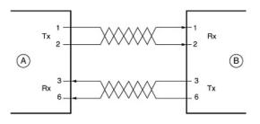
Key: A = UPLINK OR MDI PORT (as on a PC) B = Normal or MDI-X port (as on a hub or switch) 1, 2, 3, 6 = Pin numbers
