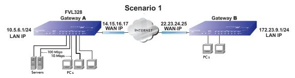
Figure 6-11: LAN to LAN VPN access from an FVL328 to an FVL328
