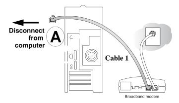
Figure 3-1: Disconnect the broadband modem
