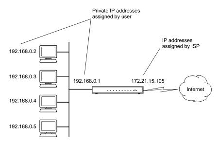
Figure 8-3: Single IP Address Operation Using NAT
