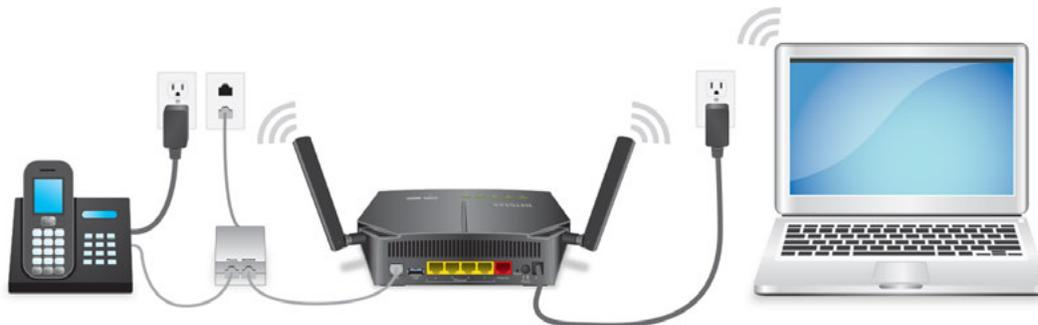
Figure 4. Modem router cabling for DSL service
