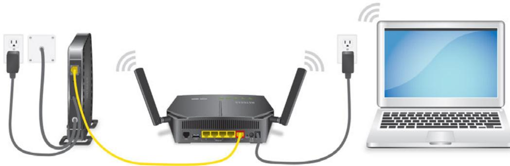
Figure 5. Modem router cabling for cable service
