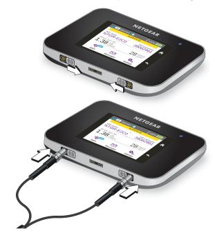
Figure 3. External antennas with TS-9 connectors
