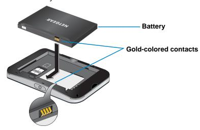
Ensure that the gold-colored contacts on the battery line up with the gold contacts on the device.
